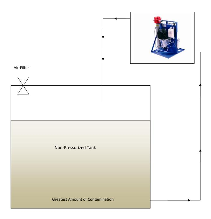
Must install PF-model on top of the tank
